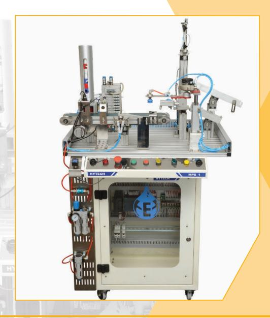
This is the first station of Hytech MPS system which is equipped with automatic loading tube. It can be connected to MPS 2.
