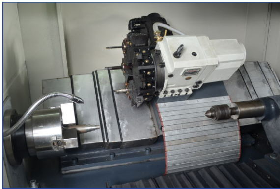
HPL 100 with Slant Bed, Hydraulic Chuck, Hydraulic Tailstock and 8 Station Production Turret
