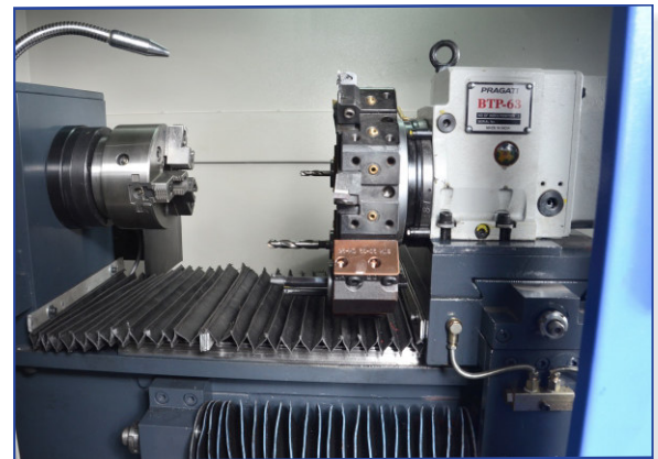
HPL 100 with Flat Bed, Hydraulic Chuck and 8 Station Production Turret
