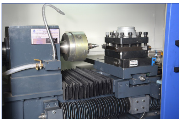
HPL 100 with Flat Bed, Manual Chuck and 4 Station Production Turret
