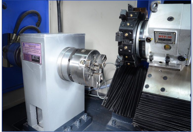
Pic : HPL 100 with Slant Bed, Hydraulic Chuck and 8 Station Production Turret
