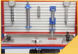
Hytech Basic Hydraulic training kit is a dual faced training kit made of heavy duty aluminum extrusions. Basic hydraulic training kit covers almost all of the commonly used conventional hydraulic valves. Hytech Training kit comes with hydraulic circuit design and
